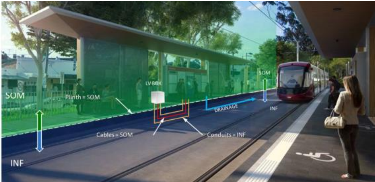
Figure 1-4: Relationship between Infrastructure Works and SOM Works
