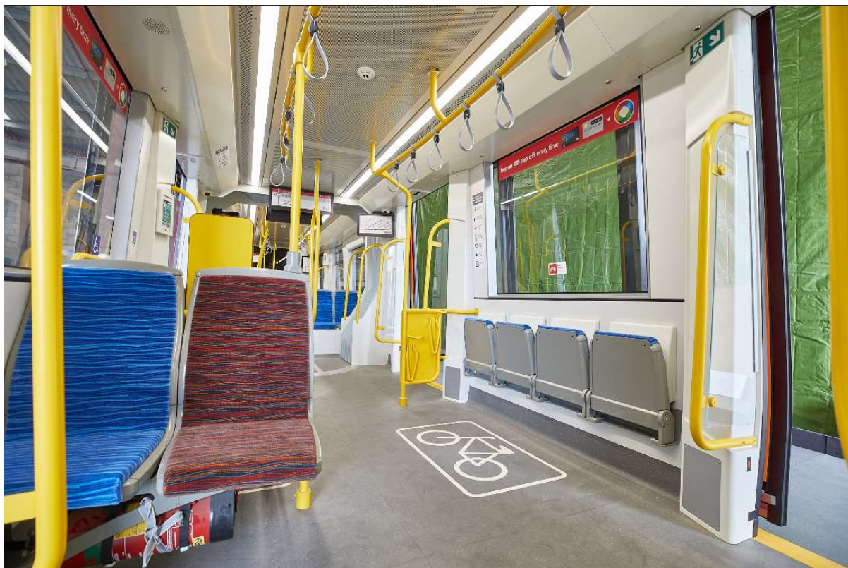
Figure 5 Photo from Saloon Mock-Up showing bicycle stowage area accommodating two bicycles in horizontal arrangement
