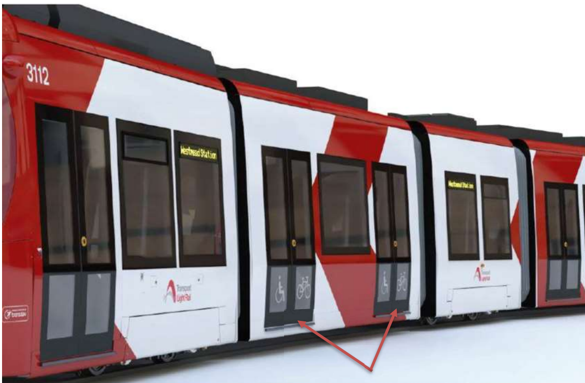
Figure 6 Example of decals that can be included on external doors of LRV cars for bike racks and wheelchair users
